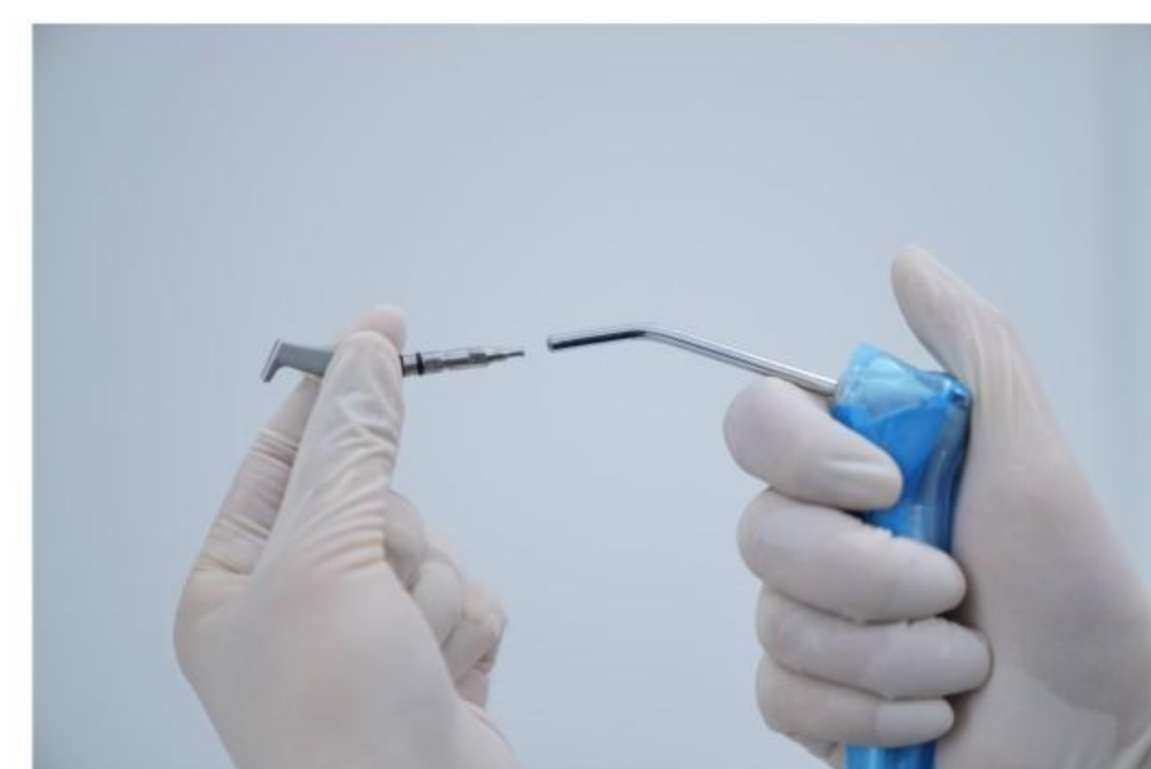
e. Use a three-way syringe to blow air to the nozzle rear end.
