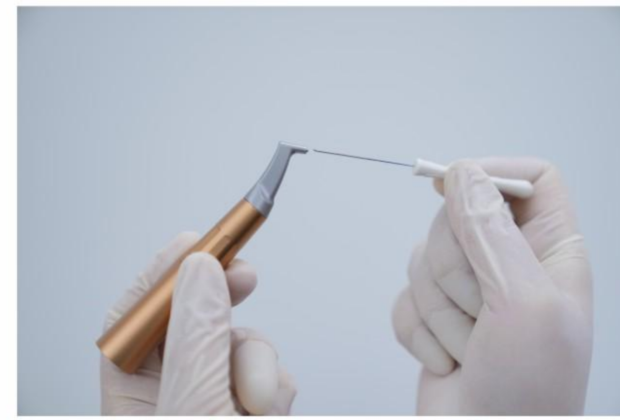
b. Unclog the nozzle central tube with the short needle. Insert, pull, and rotate several times.
