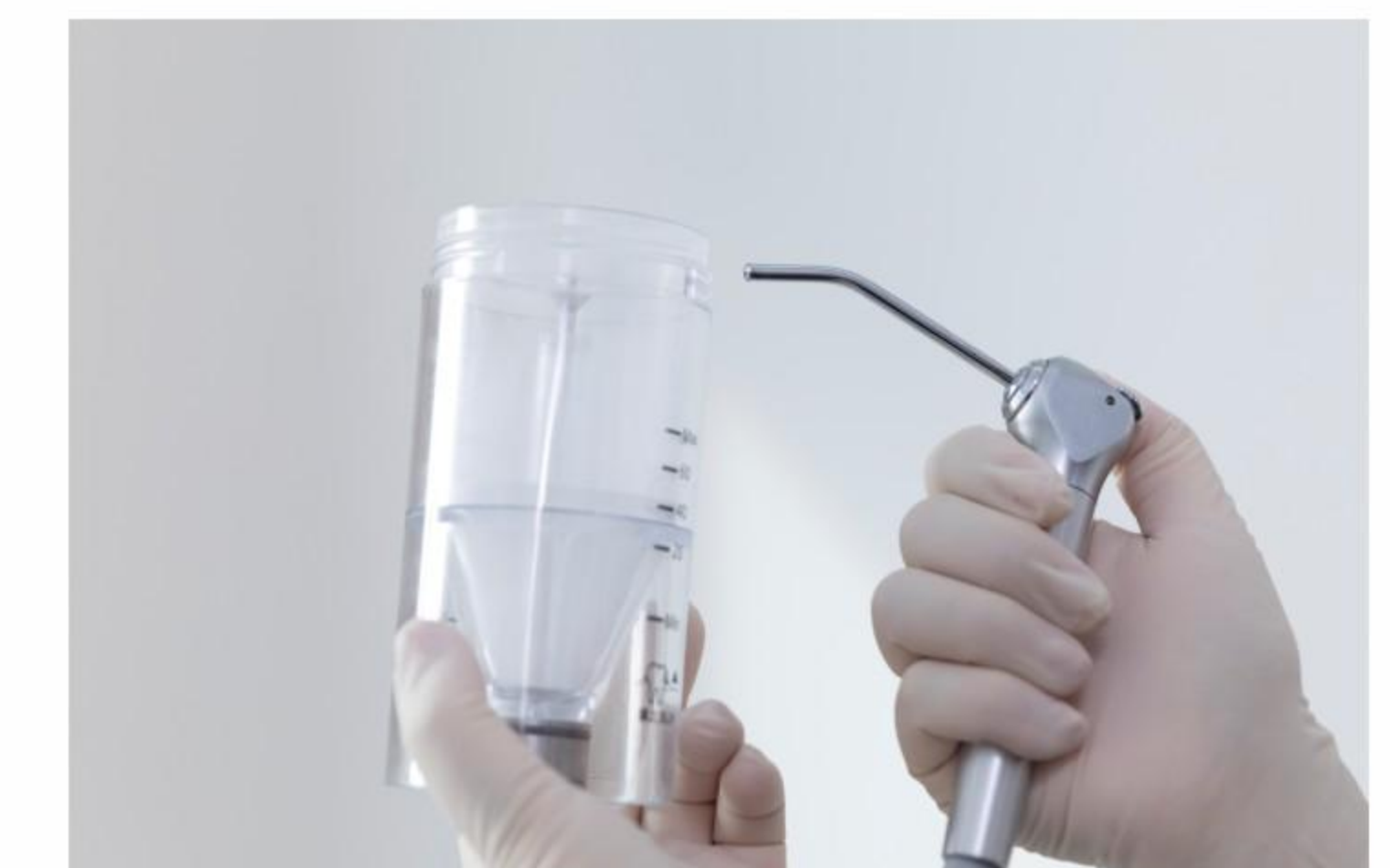
e. Use a three-way syringe to blow air to the powder tank threads.
