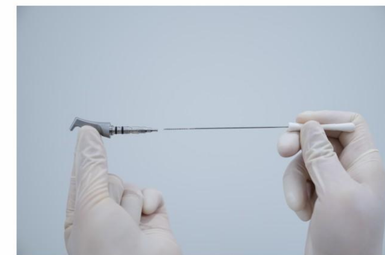
c. Unclog the nozzle rear end with the long needle. Insert, pull, and rotate several times.
