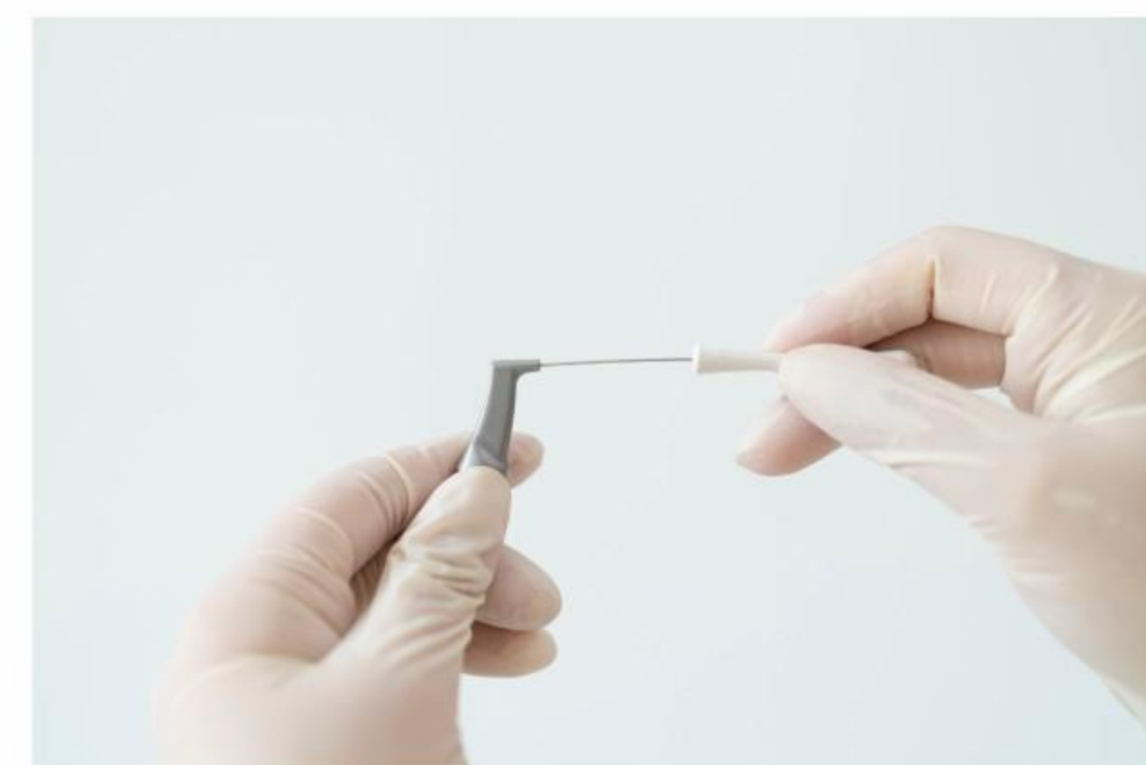
b. Unclog the nozzle front end with the short needle. Insert, pull, and rotate several times.
