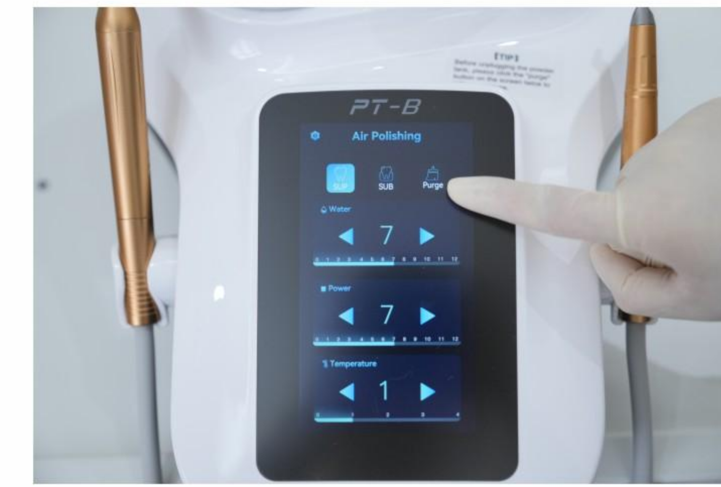
a. Touch the cleaning mode in standby mode to release the high-pressure air in the powder tank.
