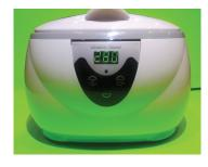
STEP 5: Set the timer of the unit to 280 seconds by pressing the 'timer' button until 280 seconds are displayed.
